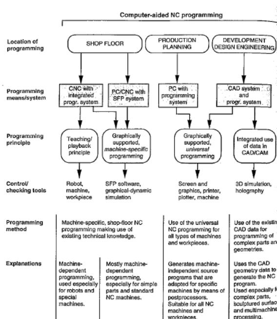
Figure 4 Interaction between programming means, programming principles, and programming methods in computer-aided programming.
