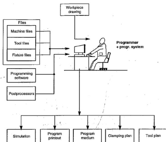
Figure 3 The principle of NC programming.
