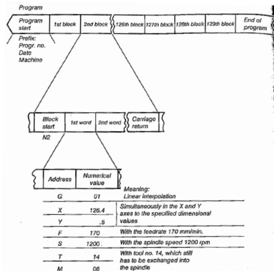
Figure 1 The basic structure of an NC program in the address format.
