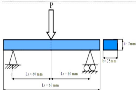
Figure 2. Testing of three point bending [7]
