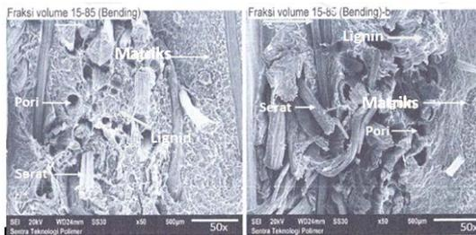
Figure 10. SEM observation of the lowest composite bending stress
