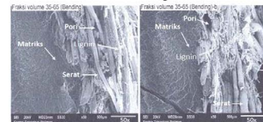
Figure 9. SEM observation of the highest composite bending stress
