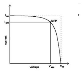
Figure 1: Solar cell characteristic curve
