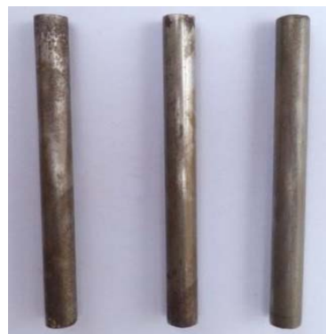
Figure 6. Reinforcing steel brand b after 45 days immersion in media seawater with addition of 2% H 2 SO 4
