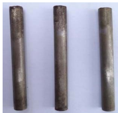
Figure 7. Reinforcing Steel Brand C After 45 days immersion of Sea water in Media With Addition of 2% H 2 SO 4
