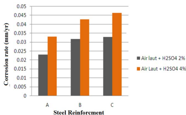
Figure 11. Brand steel reinforcement vs rate of corrosion in media immersion seawater with addition of 2% H 2 SO 4 and 4% H 2 SO 4
