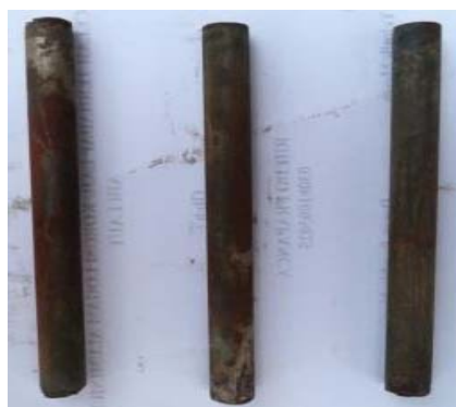
Figure 10. Reinforcing Steel Brand C After 45 days Immersion of Sea Water In Media With Addition of 4% H 2 SO 4
