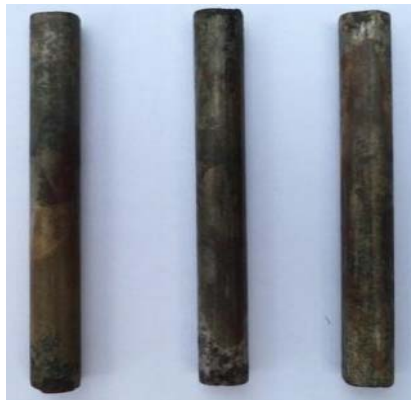
Figure 9. Reinforcing Steel Brand B After 45 Days Immersion In Media Seawater With Addition of 4% H 2 SO 4
