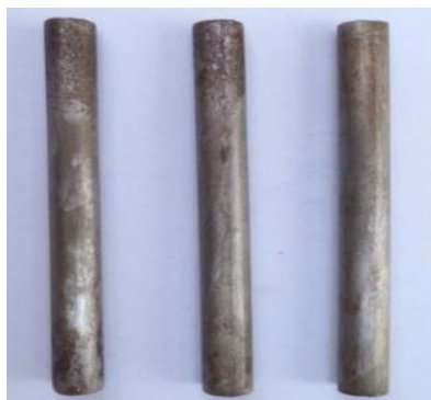
Figure 5. Reinforcing Steel Brand A After 45 Days Immersion In Media Seawater With Addition of 2% H 2 SO 4
