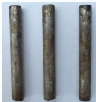
Figure 8. Reinforcing steel brand a after 45 days immersion in media seawater with addition of 4% H 2 SO 4
