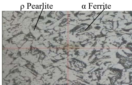
Figure 2. Metal microstructure on HAZ magnification 1000x
