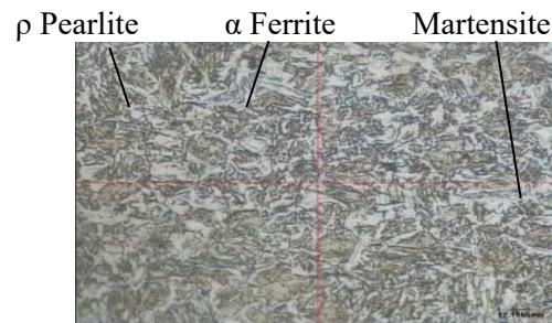
Figure 4. Main Steel microstructure in Quenching magnification 1000x
