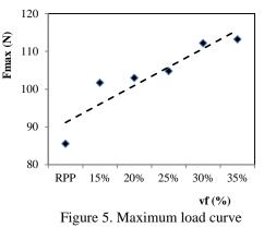
The maximum load average is highest at 35% fiber volume fraction is 113.20 N, the lowest was on 15% fiber volume fraction is 101.68 N. The increase of maximum load is caused by a perfect bond between the fiber and matrix. By the time given outside the first load of dropped out of the matrix. Followed by fiber and the fiber is gradually broken/not at once but there is still partly intact so that no visible curves drop gradually.
