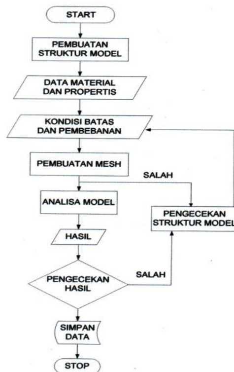
Gambar 5 Diagram alir proses analisa software Solidworks
