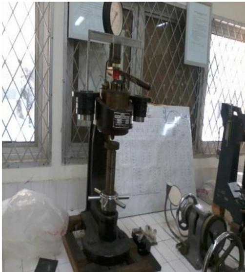
**Gambar 9** Vickers Hardness Tester
