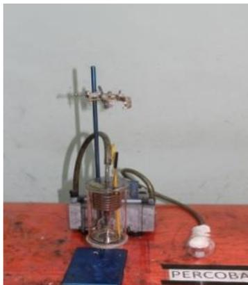
**Gambar 2.** Kalorimeter
