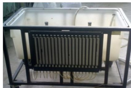
Gambar III.1. *Alat Ground-water Flow Apparatus*
