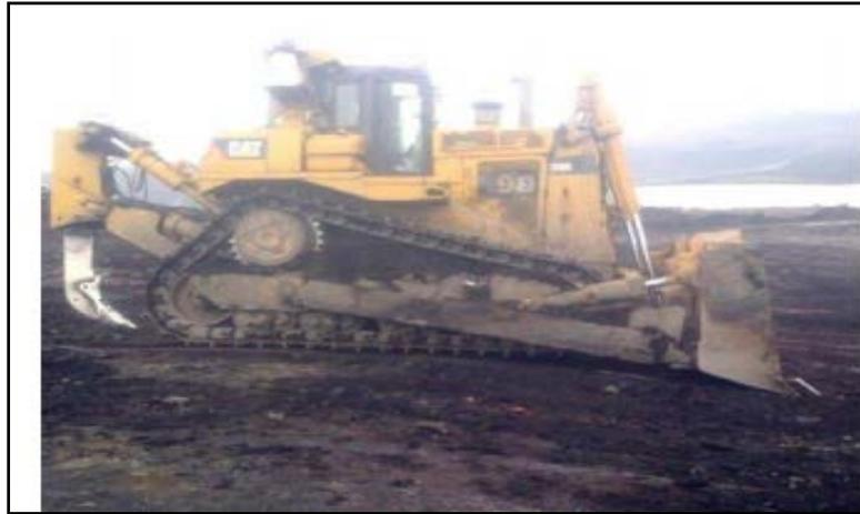
Gambar 1. Bulldozer Caterpillar D9R
