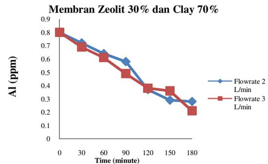
Figure 8. The decrease of Aluminium value in used oil during operation time (membrane: zeolit 30% and clay 70%)
